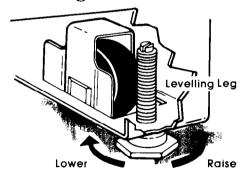
This refrigerator has 2 threaded levelling legs that are shipped in a separate package.
